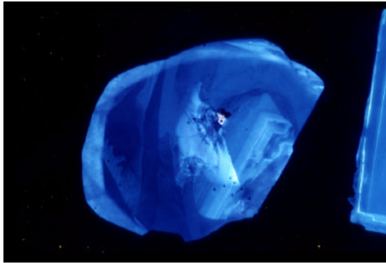
Figure 5.6_5 Cathodoluminescence of BZ252 showing a region of complex stepped growth.
