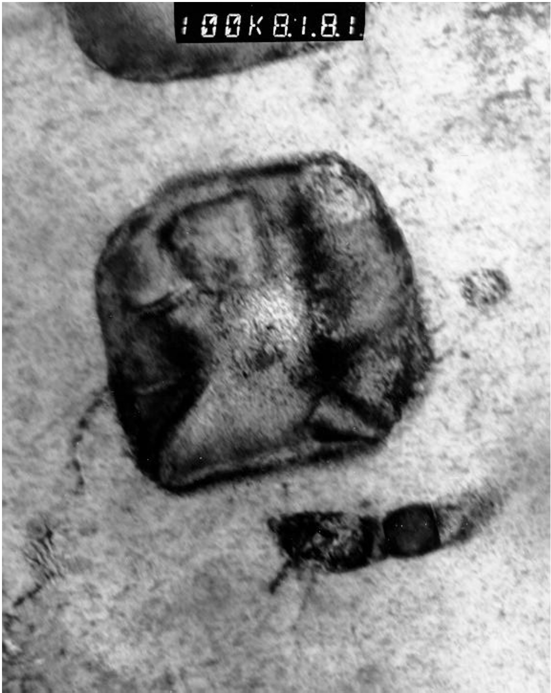
Figure 2.6_7 TEM image of a 0.4\ \mu\text{m} 'bleb' within fPer grain BZ67 showing a further 0.1\ \mu\text{m} inclusion within.
