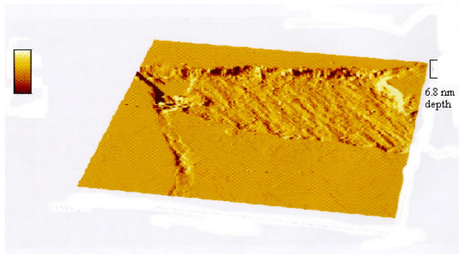
Figure 5.3_20 AFM image of BZ251B showing a regular lineation in surface topography.
