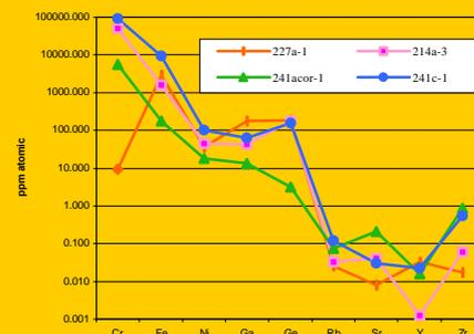
Fig. 3 Concentrations of trace elements from syngenetic inclusions of corundums in Juina diamonds
